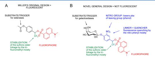
Figure 6. Design of Miller's fluorescent probe for esterases (A) and our novel design for the FDE substrate for galactosidases (B).
