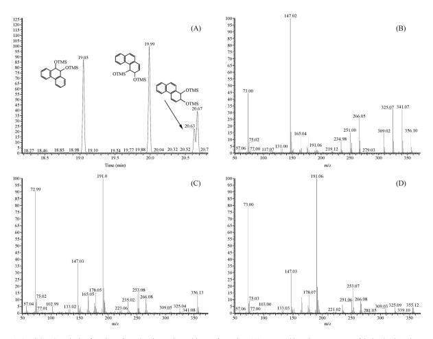
**Fig. 3** GC-MS analysis of products from the phenanthrene biotransformation. (A) Extracted ion chromatograms of derivatized products, m/z 356 [M<sup>+</sup>]; the reaction yielded 3 products in total; (B) MS of the peak of *cis*-9, 10-dihydrodiol-phenanthrene at 19.05 min; (C) MS of the peak of *cis*-3, 4-dihydrodiol-phenanthrene at 19.99 min; (D) MS of the peak of *cis*-1,2-dihydrodiol-phenanthrene at 20.63 min.
